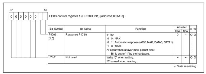
Fig. 64 Structure of EP03 control register 1
