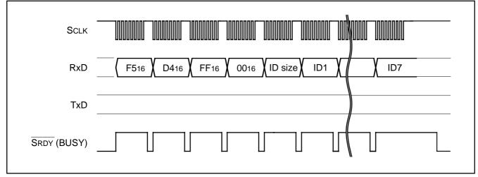
Fig. 132 Timing for ID check
