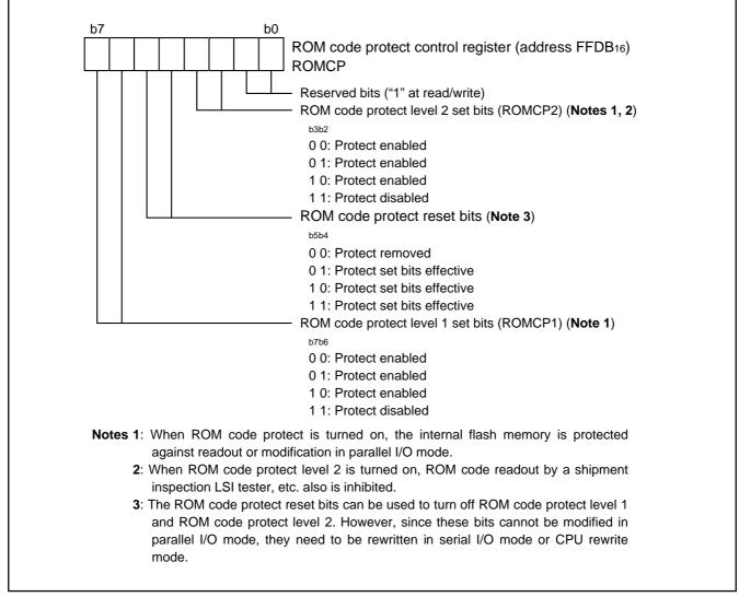
Fig. 121 Structure of ROM code protect control register
