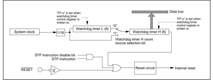
Fig. 104 Block diagram of Watchdog timer
