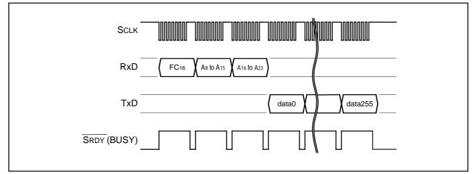
Fig. 131 Timing for Boot ROM area output
