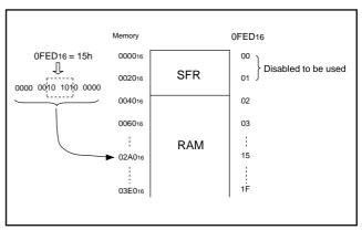
Fig. 26 Example setting of buffer area beginning address
