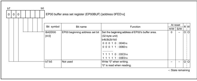
Fig. 44 Structure of EP00 buffer area set register
