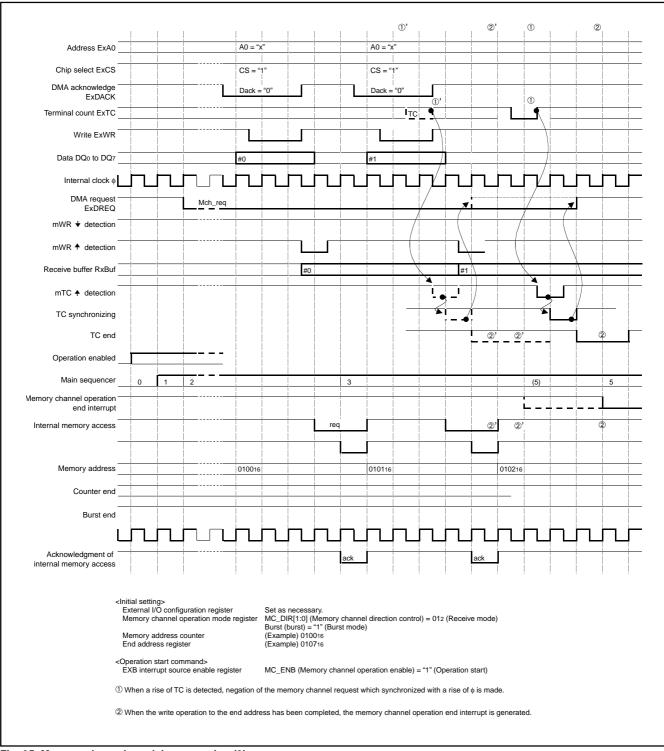
Fig. 95 Memory channel receiving operation (3)
