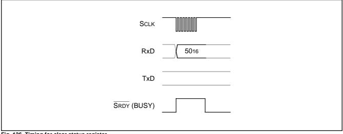
Fig. 126 Timing for clear status register
