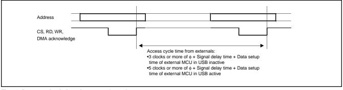
Fig. 73 Data transfer timing of memory channel
