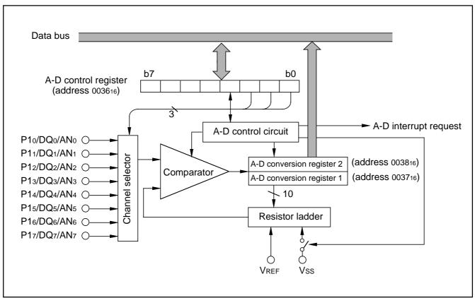
Fig. 103 A-D converter block diagram
