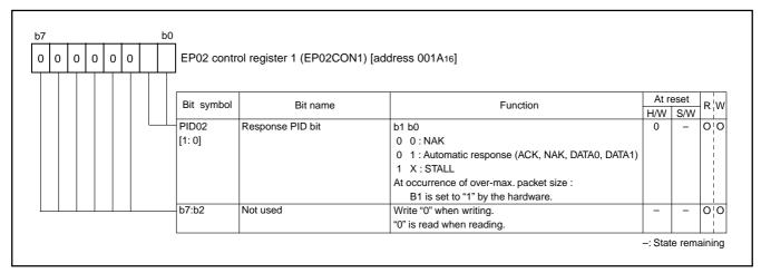
Fig. 55 Structure of EP02 control register 1
