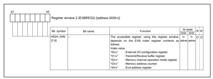
Fig. 82 Structure of Register window 2
