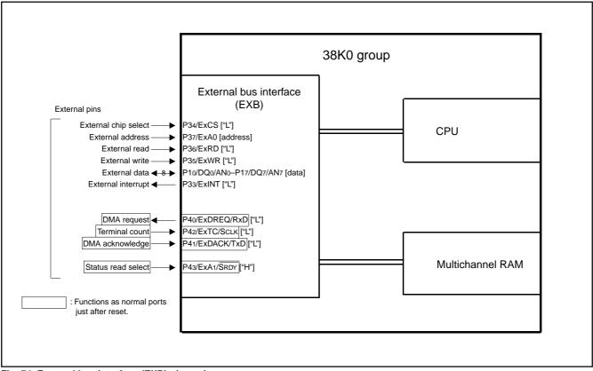
Fig. 74 External bus interface (EXB) pin assignment
