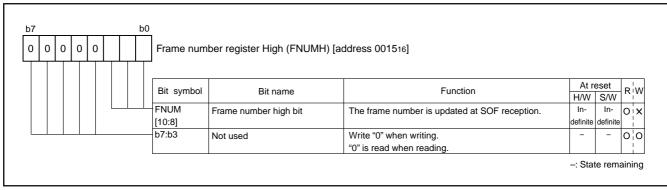
Fig. 34 Structure of Frame number register High
