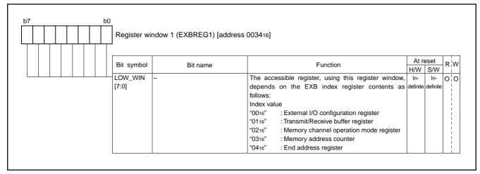
Fig. 81 Structure of Register window 1
