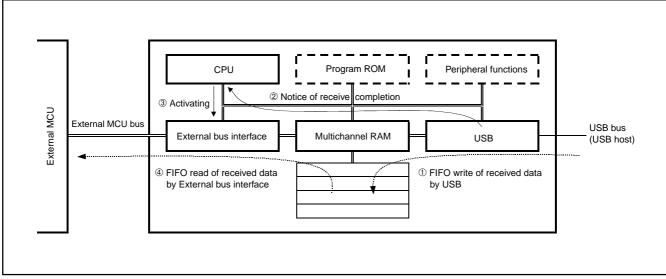
Fig. 100 Multichannel RAM operation example
