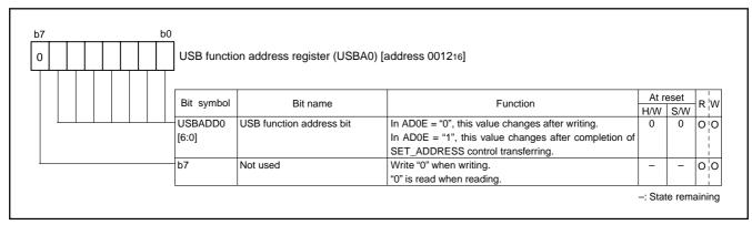
Fig. 32 Structure of USB function address register
