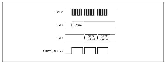
Fig. 125 Timing for reading status register
