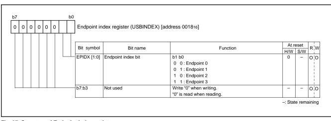
Fig. 37 Structure of Endpoint index register
