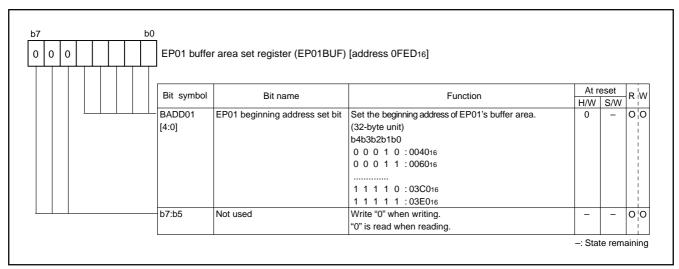
Fig. 53 Structure of EP01 buffer area set register
