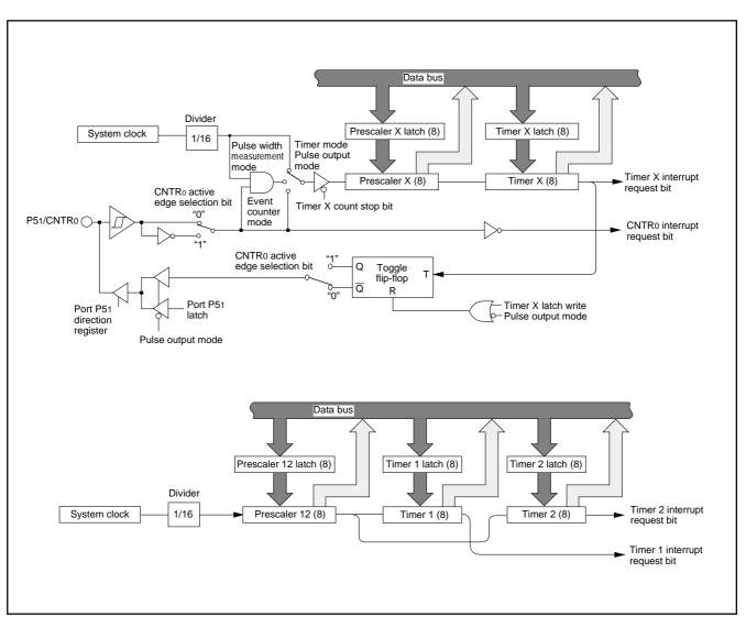
Fig. 17 Timer block diagram
