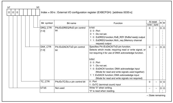
Fig. 84 Index00[high]; Structure of External I/O configuration register
