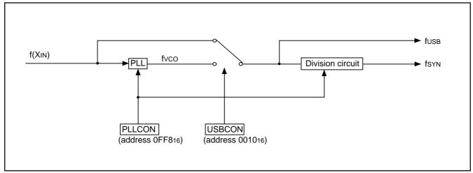
Fig. 108 Block diagram of PLL circuit
