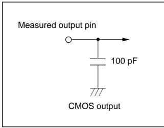
Fig. 137 Output switching characteristics measurement circuit
