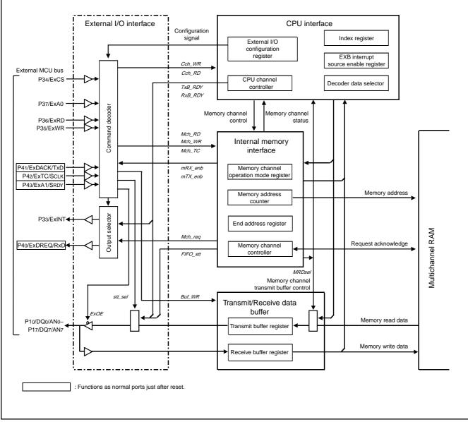
Fig. 75 Block diagram of external bus interface (EXB)
