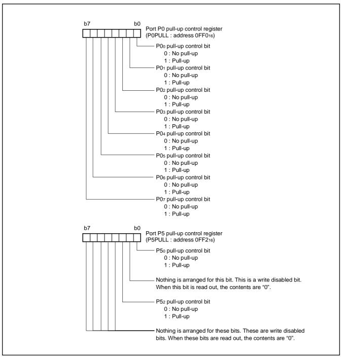
Fig. 12 Structure of port I/O-related registers
