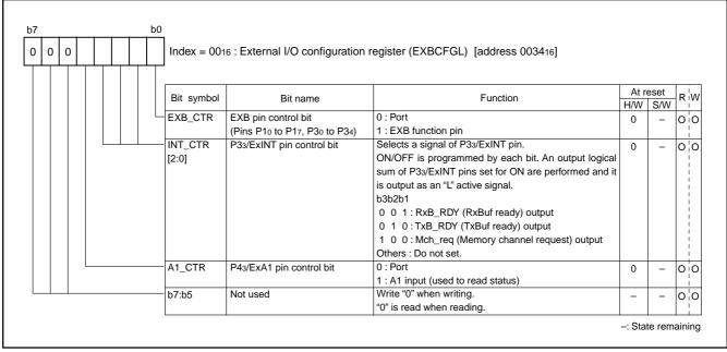
Fig. 83 Index00[low]; Structure of External I/O configuration register
