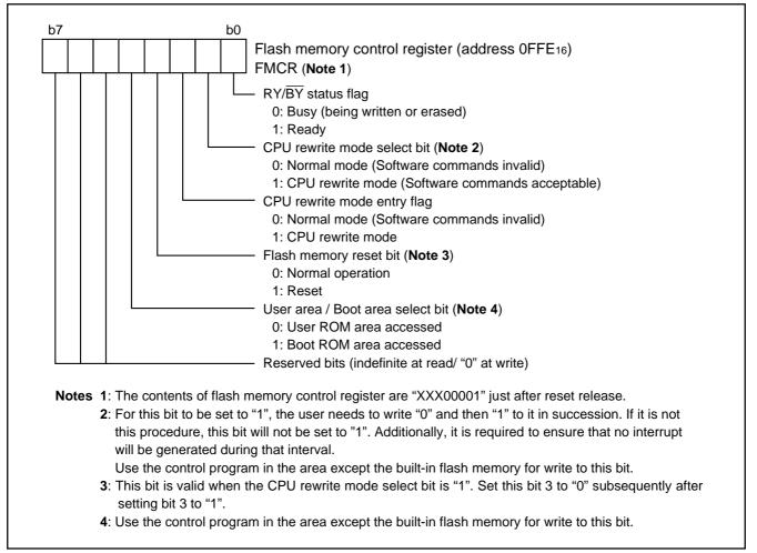
Fig. 116 Structure of flash memory control register
