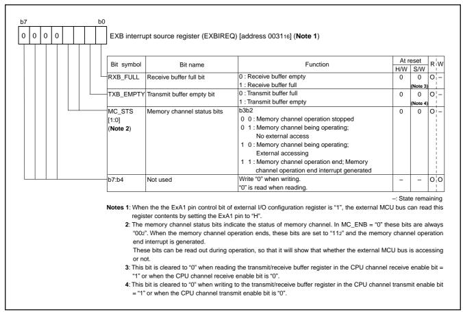
Fig. 79 Structure of EXB interrupt source register
