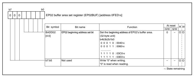
Fig. 62 Structure of EP02 buffer area set register
