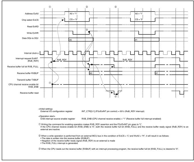
Fig. 91 CPU channel receiving operation
