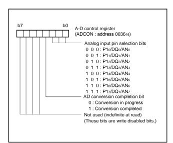
Fig. 101 Structure of A-D control register
