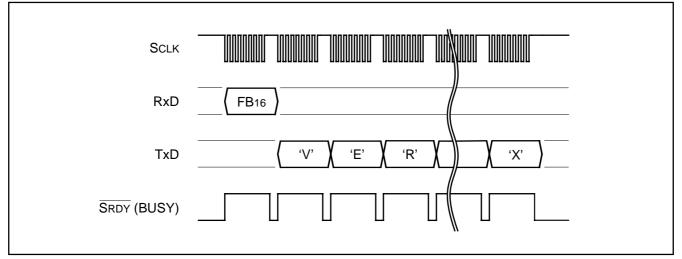
Fig. 130 Timing for version information output
