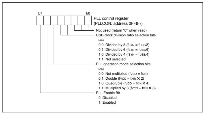
Fig. 109 Structure of PLL control register
