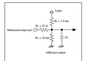
Fig. 139 USB output switching characteristics measurement circuit (2) for D0+
