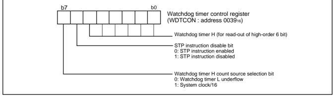
Fig. 105 Structure of Watchdog timer control register
