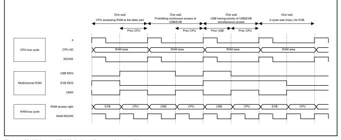
Fig. 99 Multichannel RAM timing diagram (one wait)
