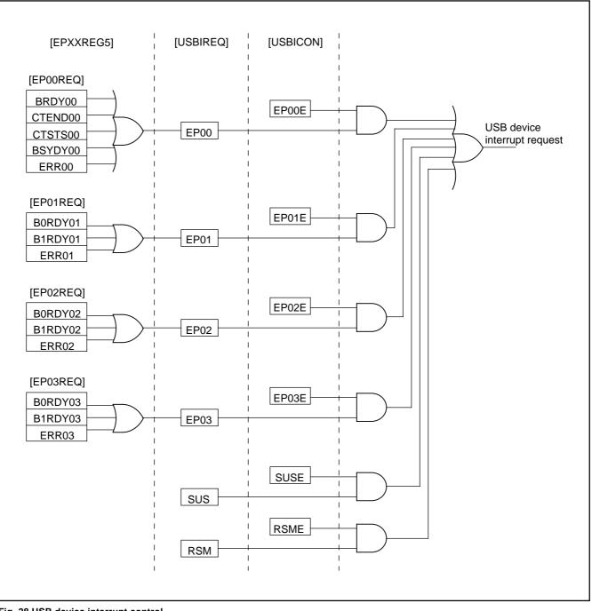
Fig. 28 USB device interrupt control
