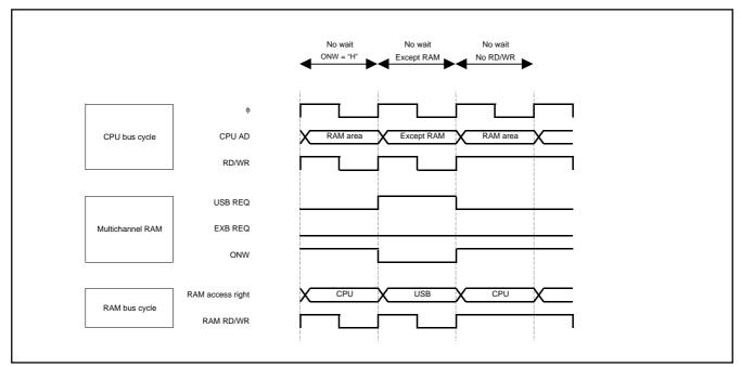
Fig. 98 Multichannel RAM timing diagram (no wait)
