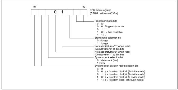
Fig. 7 Structure of CPU mode register
