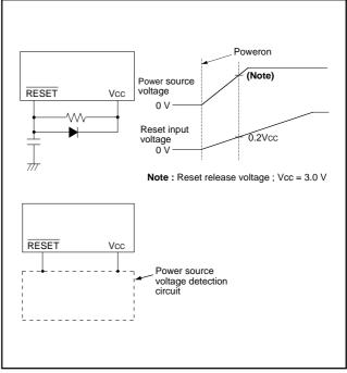
Fig. 106 Example of reset circuit
