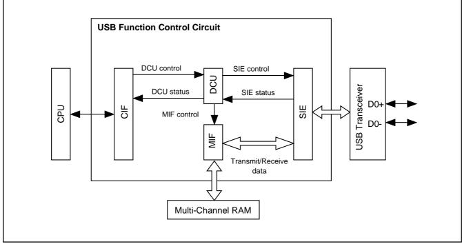
Fig. 24 USB Function Control Circuit (USBFCC) block diagram
