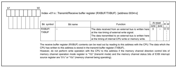
Fig. 85 Index01[low]; Structure of Transmit/Receive buffer register
