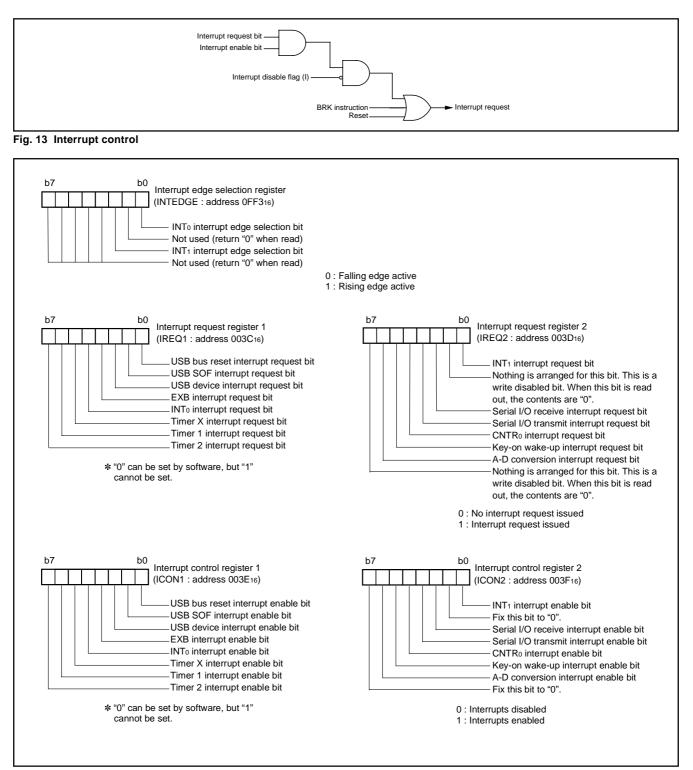
Fig. 14 Structure of interrupt-related registers
