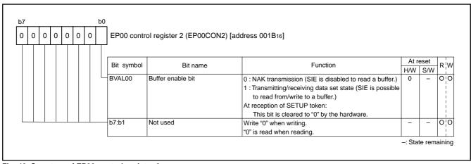
Fig. 40 Structure of EP00 control register 2
