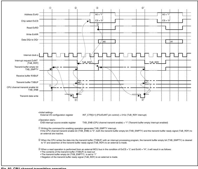
Fig. 92 CPU channel tranmitting operation
