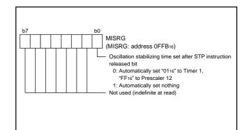
Fig. 112 Structure of MISRG
