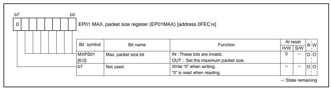
Fig. 52 Structure of EP01 MAX. packet size register
