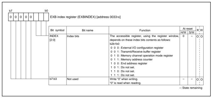
Fig. 80 Structure of EXB index register
