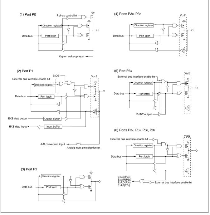
Fig. 10 Port block diagram (1)
