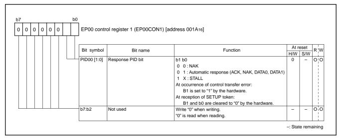
Fig. 39 Structure of EP00 control register 1
