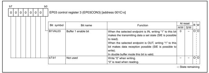
Fig. 66 Structure of EP03 control register 3
