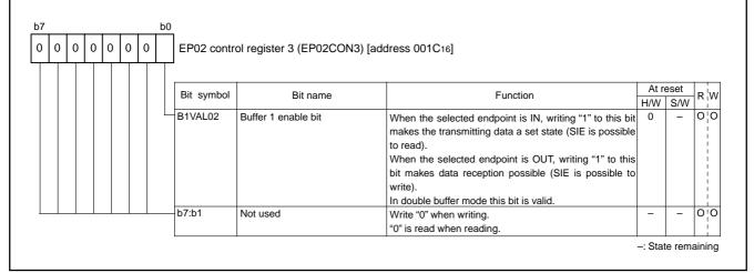
Fig. 57 Structure of EP02 control register 3
