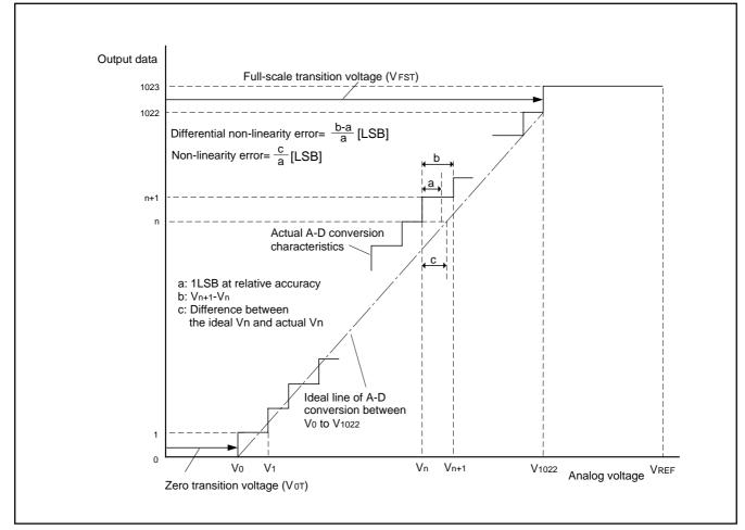
Fig. 136 Definition of A-D conversion accuracy
