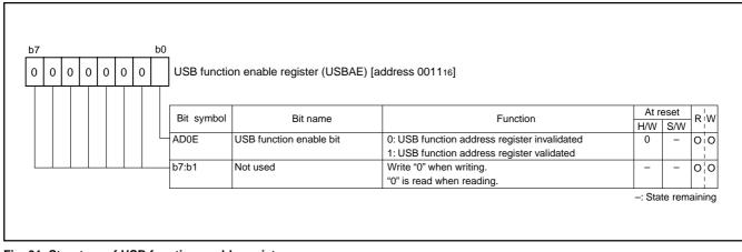
Fig. 31 Structure of USB function enable register
